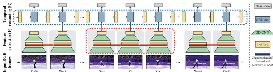
Fig. 2: **Overview of E2E-Spot.** RGB video frames are first input to a local spatial-temporal feature extractor  $F$  (a RegNet-Y [43] with GSM [54]) to produce a feature for each frame that captures subtle differences and motion across neighboring frames (red dotted box). The feature sequence is then processed by a sequence model  $G$ , which builds a long-scale temporal context (blue dotted box; one direction drawn) and outputs a class prediction for every frame.
